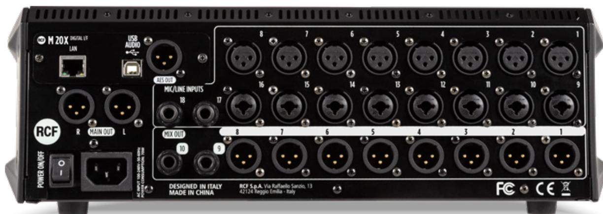
On the M 20X rear panel, 8 Mic inputs equipped with XLR connector and 8 Mic/Line inputs with COMBO connectors are available, with two additional TRS jacks line inputs. The MIX output section includes 8 male XLR and 2 TRS jacks on which all the internal audio output paths can be routed. A pair of male XLR, preassigned to the Main Mix output, and an assignable
